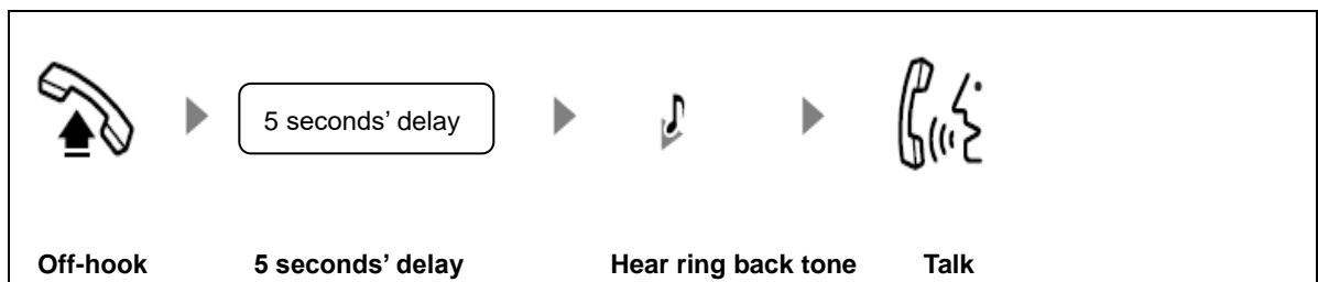
Figure 2-7 Hotline with delay
