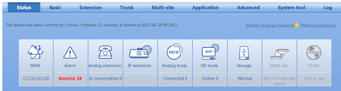
Figure 2-91 Running status interface
