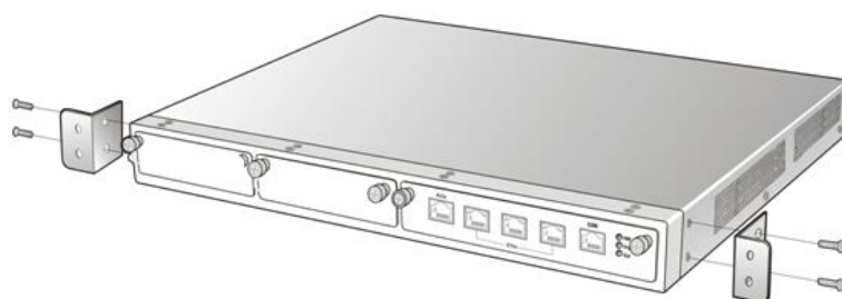
Figure 2-1 Installation of SX1000 L-shape brackets
